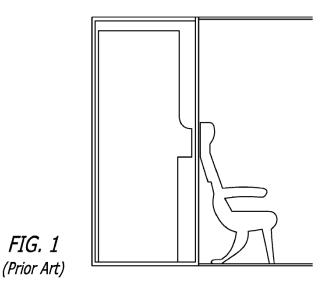
Figure 1, reproduced above, illustrates "a prior art installation of an aircraft lavatory immediately aft of and adjacent to an aircraft passenger seat." Ex. 1001, 4:11–13. In the depiction of the prior art in Figure 1, a forward wall of the lavatory (double-lined structure immediately aft of seat) is flat and in a vertical plane.
