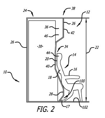
Figure 2, reproduced above, illustrates enclosure 10, such as a lavatory, positioned aft of aircraft cabin 12. Ex. 1001, 4:22–27. The lavatory has walls that define interior lavatory space 30. *Id.* at 4:33–36. Forward wall 28 of the lavatory is described as "substantially not flat in a
