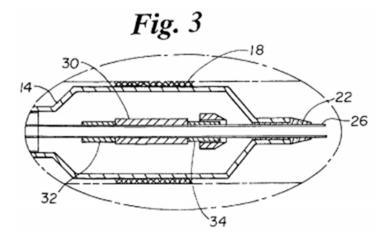
Figure 3 depicts an enlarged cross-sectional view of the distal end of catheter 12, with balloon 14 and stent 18 in expanded states. *Id.* at 2:20–23. As shown in Figure 3, "a mounting body 30 . . . is included inside balloon 14 to provide a cushion and/or substrate of enlarged diameter relative to the stent shaft to support and hold the stent and secure it during crimping and
