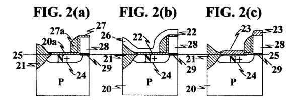
Figures 2(a), 2(b), and 2(c) are cross-sectional views of a method of forming a refractory metal silicide at the surface of an active region of a transistor. *Id.* at 2:56–58.
