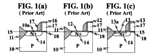
Figures 1(a), 1(b), and 1(c) are cross-sectional views of a prior art method of forming a refractory metal silicide at the surface of an active region of a transistor. *Id.* at 2:53–55.
