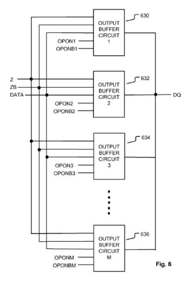
As shown in Figure 6 above, the output buffers receive control-input signals (OPON1–OPONM and OPONB1–OPONBM). *Id.* at 8:35–38. These control-input signals can enable some output buffer circuits and disable
