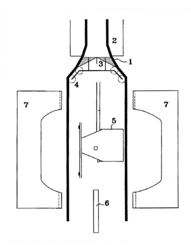
The figure depicts "an extrusion blow-[molding] machine with continuous extrusion used for producing motor-vehicle fuel tanks." *Id.* at 2:41–45. The circular die of extrusion head 2 produces tubular
