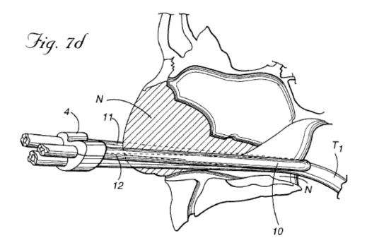
Figure 7d depicts flexible member 10 looped posteriorly around nasal septum N and magnetic probe 20 separated from end potion 12. *Id.* at 6:64–7:2. Receiver 24<sup>2</sup> is secured to end portions 11, 12 of flexible member 10 and to nasal tube T<sub>1</sub>, which is inserted into one of the patient's nares. *Id.* at 7:3–13, Fig. 7d.
