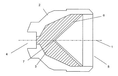
Figure 1 is a cross-sectional view of a shaped charge that includes a substantially cylindrical housing 2, a liner 6 that fits closely in the open end
