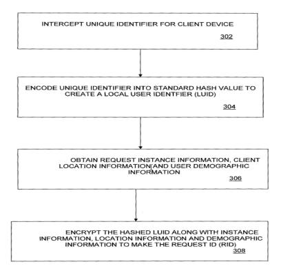
Figure 3 above is a flowchart illustrating a method of generating a request identifier. *Id.* at 4:5–6. At block 302, tag processor 206 intercepts the device identifier (e.g., the MAC address of client device 202). *Id.* at 8:30–34. At block 304, tag processor 206 encodes the device identifier to
