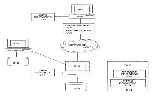
Figure 2 above illustrates a client-server network including a network tagging component. *Id.* at 7:53–54. According to the '747 patent, Figure 2 shows a standard Internet Protocol ("IP") based access system in which
