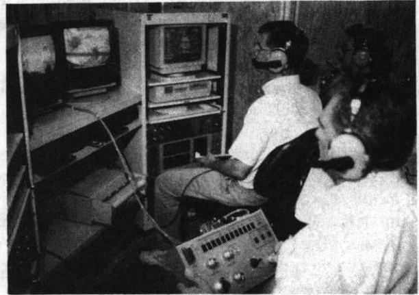
Figure 3 The Cypher aircraft operator console provides an integrated display of the external situation.
