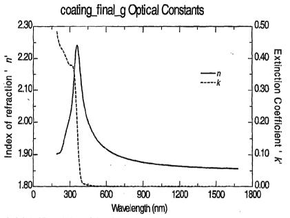
n,k of 300A of ZnO:Al2O3 on soda lime glass. Denton coater
