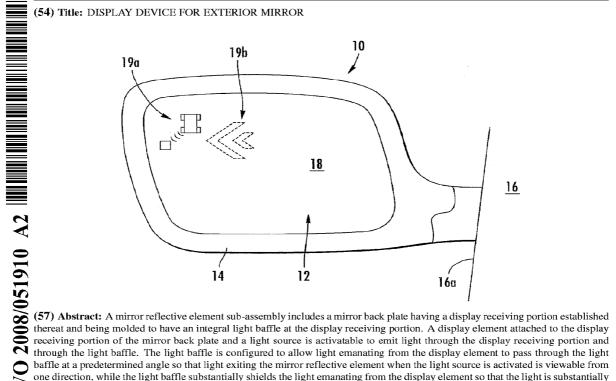
baffle at a predetermined angle so that light exiting the mirror reflective element when the light source is activated is viewable from one direction, while the light baffle substantially shields the light emanating from the display element so that the light is substantially non-viewable from another direction.
