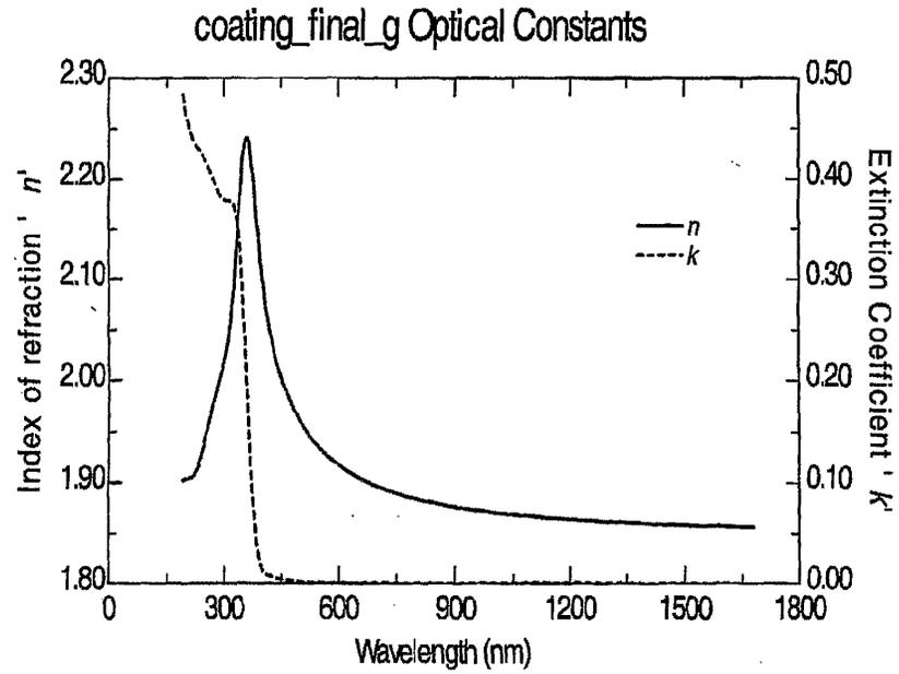
n,k of 300Å of ZnO:Al<sub>2</sub>O<sub>3</sub> on soda lime glass. Denton coater
