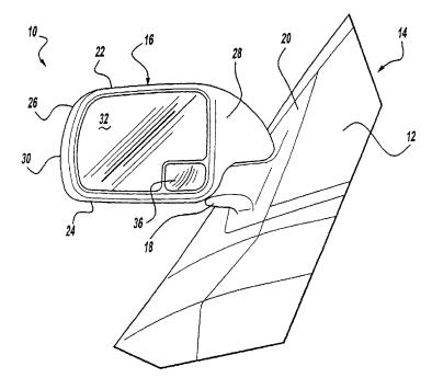
(57) Abstract: A mirror assembly (10) in which a mirror housing (16) and multi-function backing plate (34) provides various useful functions. The multi-function backing plate supports not only a conventional reflective element (32) but also supports a wide angle reflective element (36). The multi-function backing plate further supports an indicator light assembly (96) so that the mirror assembly can provide an indicator light function.
