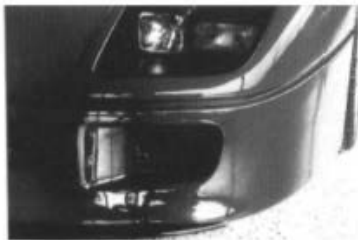
5.19 Front spoiler of Ferrari F40 in a polyurethane integral skin system (courtesy Dow Plastics).
