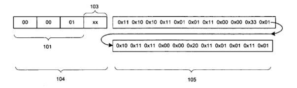
Figure 1 depicts the block diagram of encapsulated video payload 100 with a delimiter.
