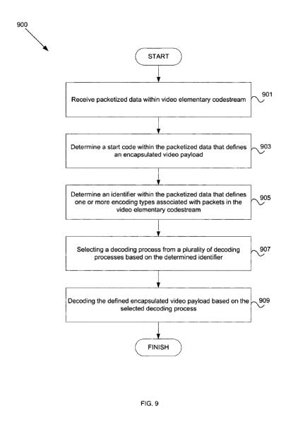
Figure 9 depicts a method for decoding an encoded video stream.
