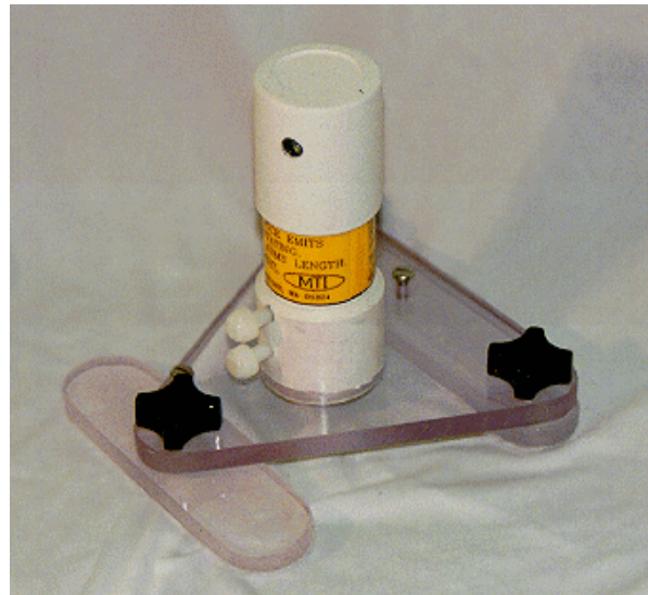
Figure 6.19: A single STROAB beams a vertically spread laser signal while rotating at 3,000 rpm. (Courtesy of, MTI Research Inc.)
