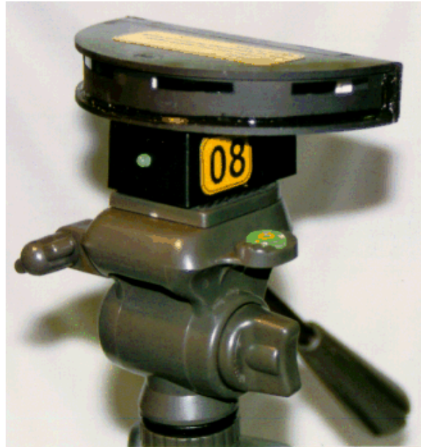
Figure 6.20: Stationary NOADs are located at known positions; at least two NOADs are networked and connected to a PC. (Courtesy of MTI Research, Inc.)
