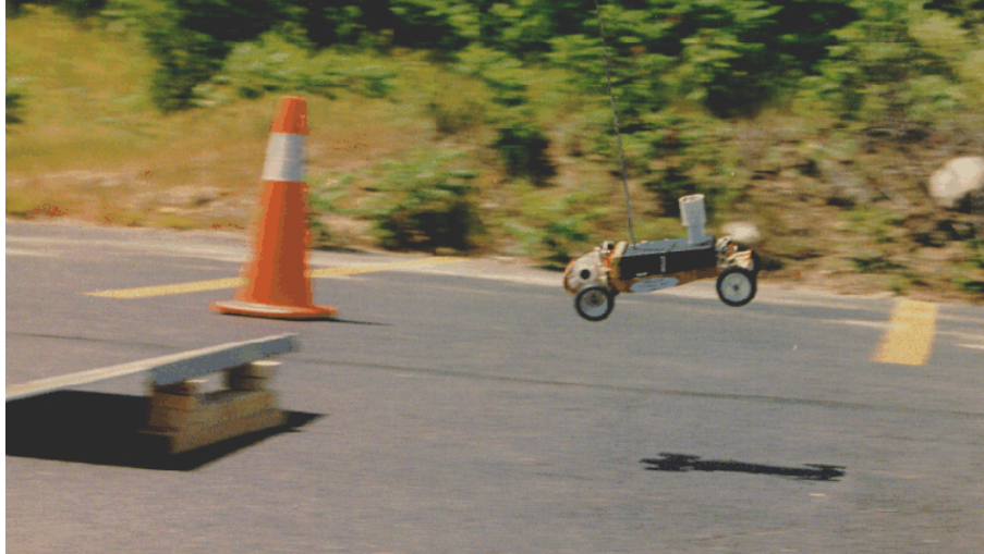
Figure 6.22: MTI's Scooter zips through a race course; tight close-loop control is maintained even in mid-air and at speeds of up to 6.1 m/s (20 ft/s).
