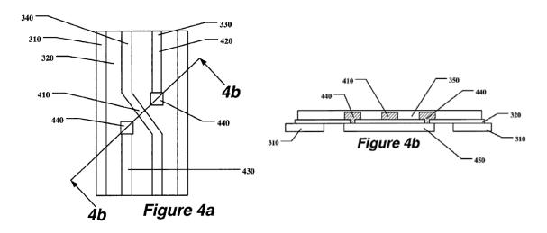
Figures 4a and 4b "provide an illustration of a laminated suspension with a crossover electrical trace." *Id.* at 3:15–17. Figure 4a shows the top view "of a laminated suspension using a crossover feature of the present invention," while Figure 4b illustrates a cross-sectional view of the same structure. *Id.*
