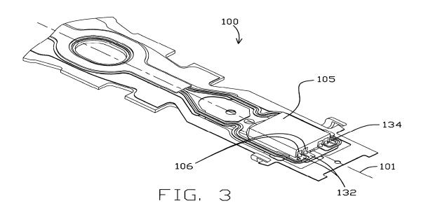
Figure 3, reproduced above, depicts head suspension 100, head slider 105, head slider bonding pads 106, trace bonding pads 132, and solder balls 134. Ex. 1001, 3:28–43. Solder balls 134 are applied at the juncture of head slider bonding pads 106 and trace bonding pads 132 to electrically connect head slider 105 to traces 130. *Id.* at 3:43–45. More specifically, the
