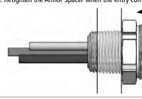
Finally, holding the cable central in the gland, tighten the and the seal to engage the cable jacket. Do not over tighte close face to face.
