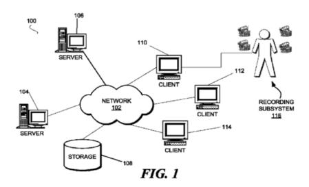
Figure 1 depicts a network of data processing systems in which illustrative embodiments may be implemented. *Id.* at 3:53–55. Data processing system 100 contains network 102, servers 104, 106, storage unit 108, clients 110, 112, 114, and recording subsystem 116. *Id.* at 3:55–4:27.
