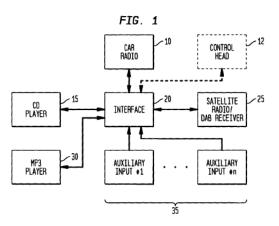
Figure 1 illustrates an embodiment integrating a car stereo with a CD player, a MP3 player, and a satellite radio or DAB receiver, as well as a number of auxiliary input sources. *Id.* at 3:12–13, 5:14–27.
