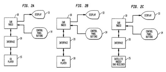
Figures 2A–C illustrate embodiments in which a car stereo is integrated with a CD player (Figure 2A), an MP3 player (Figure 2B), and a satellite radio or DAB receiver (Figure 2C). *Id.* at 3:14–23.
