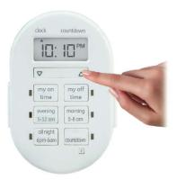
The user interface is the set of control buttons and the display of the timer, as shown in the picture accompanying step 2. The GE MyTouchSmart<sup>TM</sup> Indoor Plug-In Digital Timer therefore has an actuator on the interface enabling selection of a time. These same actuators are used both to set the clock time and to set the program times for the user programs.
