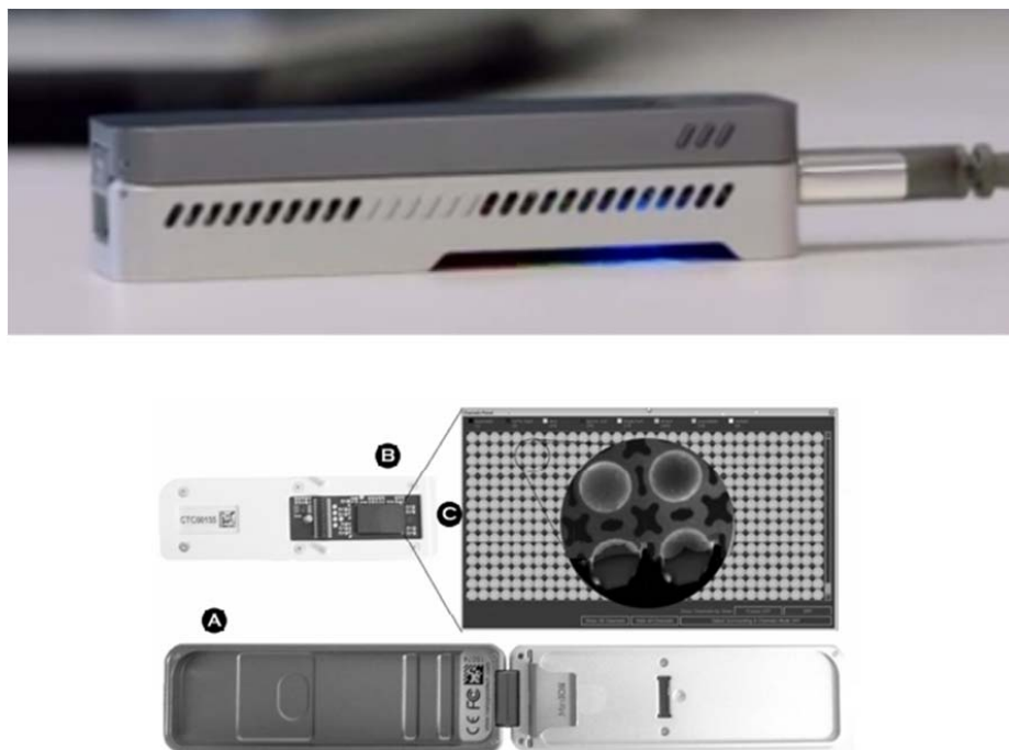
Figure 4. (A) MinION Mk1 (B) flow cell (C) nanopore array (Individual nanopore cells reproduced, modified, with permission from Oxford Nanopore).
