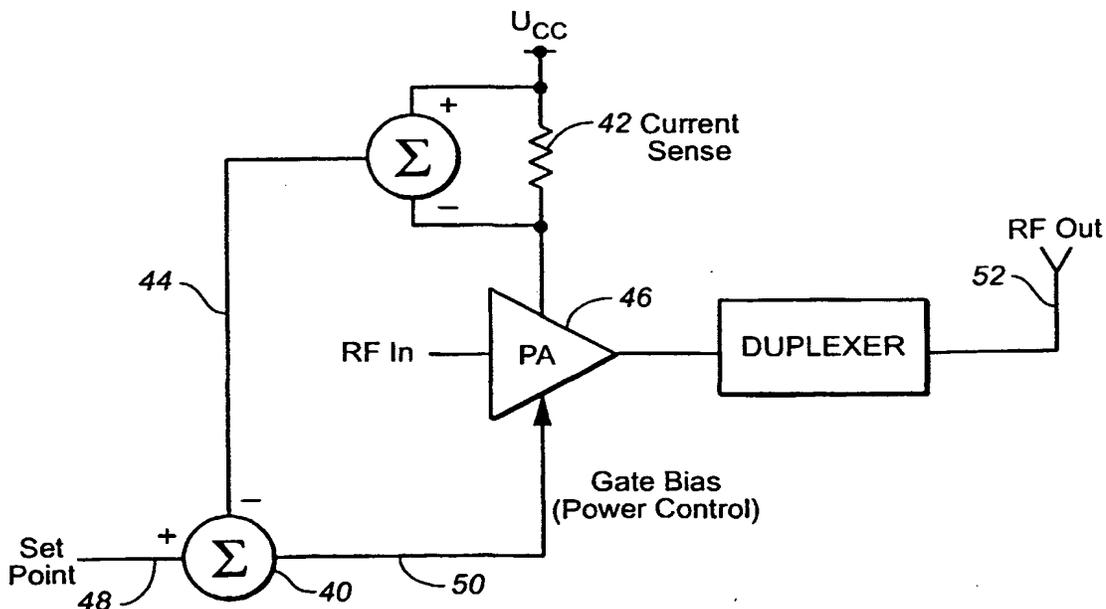
(57) Abstract: A hand-held, PCMCIA cellular radio modem card is described which uses a non-standard power output level. The non-standard power output is defined as the maximum RF power attainable such that the current drawn by the power amplifier does not exceed 400 mA. This definition permits the use of the wireless modem inside hand-held computing devices without the use of an additional battery pack extension.
