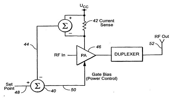
(57) Abstract: A hand-held, PCMCIA cellular radio modem card is described which uses a non-standard power output level. The non-standard power output is defined as the maximum RF power attainable such that the current drawn by the power amplifier does not exceed 400 mA. This definition permits the use of the wireless modem inside hand-held computing devices without the use of an additional battery pack extension.
