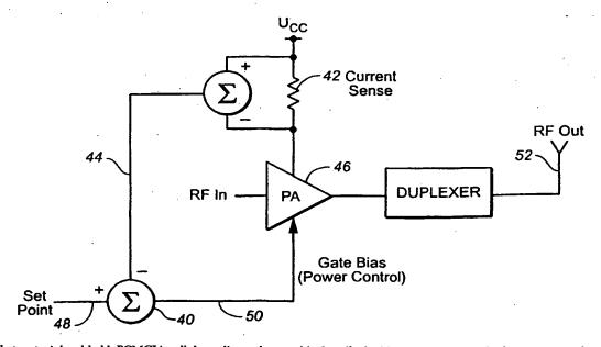
(57) Abstract: A hand-held, PCMCIA cellular radio modern card is described which uses a non-standard power output level. The non-standard power output is defined as the maximum RF power attainable such that the current drawn by the power amplifier does not exceed 400 mA. This definition permits the use of the wireless modern inside hand-held computing devices without the use of an additional battery pack extension.
