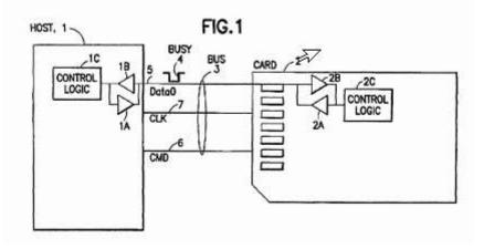
Figure 1 is a block diagram showing a first unit coupled to a second unit over a bus. *Id.* at 3:39–40. The first unit is host 1, and the second unit is memory card 2. *Id.* at 3:46–47. Connecting host 1 and memory card 2 is bus 3 that includes data line 5, command line 6, and clock line 7. *Id.* at 3:46–50. Figure 1 illustrates busy signal 4 associated with data line 5. *Id.* at
