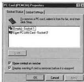
Figure 13.5 A computer with PC Card support enabled and one of its two PC Card slots in use.
