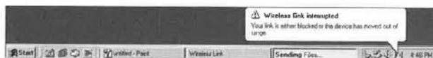
Figure 13.21 Wireless Link alerts you to a break in transmission, which could be caused by stray light or physical interference with the IR signal.
