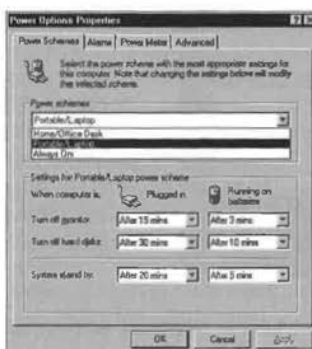
Figure 13.3 Use the Power Options Properties dialog box to control the power management settings.
