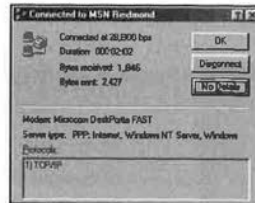
Figure 22.20 To eliminate the display of connection information in the bottom of this status dialog box, click the No Details button.
