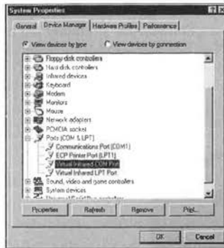
Figure 13.16 The Virtual Infrared COM and LPT ports are used for infrared file transfers and printing.
