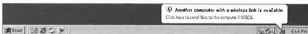
Figure 13.19 When you see this message, Wireless Link has made con- tact with another wireless device.
