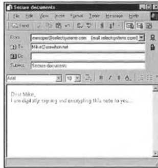
Figure 26.28 A digitally signed and encrypted message—just look for the wax-seal and padlock icons to the right of the address lines.
