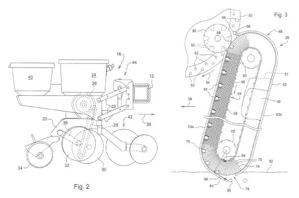
Figure 2 illustrates a side view of row unit 16 of a seeding machine, including seed hopper 24, seed meter 26, and seed delivery system 28 (shown in more detail in Figure 3). *Id.* at 2:49–52, 3:16–29. Seed stored in seed hopper 24 is provided to seed meter 26 and carried by delivery system 28 into a planting furrow or trench first formed by furrow openers 30 and then closed over the seed by closing wheels 34. *Id.* at 3:23–30.
