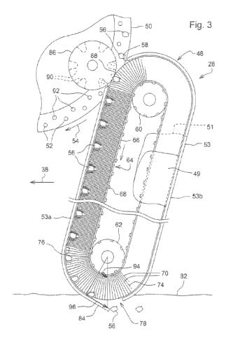
Figure 3 depicts an enlarged side view of a seed delivery system of one embodiment of the invention. Ex. 1001, 2:48–49.
