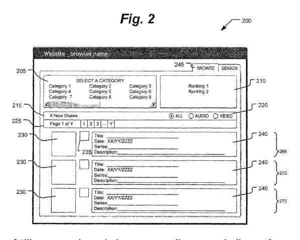
Figure 2 "illustrates an electronic document according to an embodiment of the present invention." *Id.* at 3:22–23. Web page 200 "aggregates audio and/or video content for presentation to users of computers 20." *Id.* at 5:4–6. It displays a row for each of three presentations 265, 270, and 275, each row including particular content graphics 230, particular content information 240, and indicator 235. *Id.* at 5:16–20. "A user may select such a
