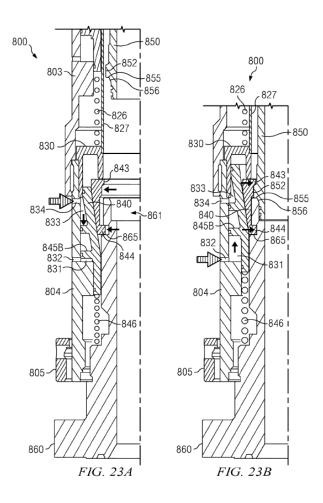
Figures 23A and 23B are partial section views of a lower end of a first wedge seal embodiment in an unlocked position and a locked position, respectively. *Id.* at 10:6–8. Wedge seal assembly 800 includes adapter 850, lower wedge 840, and lower wedge receptacle 845. *Id.* at 21:17–34. The wedge seal assembly is used to create a high pressure seal between the adapter and receptacle 860. *Id.* at 20:63–21:11; *see also id.* at 13:8–30 (discussing the high pressure seal).
