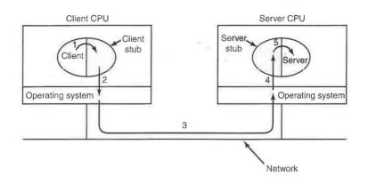
Figure 6-24. Steps in making a remote procedure call. The stubs are shaded.
