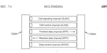
Figure 7-66. Logical channels between the caller and callee during a call.
