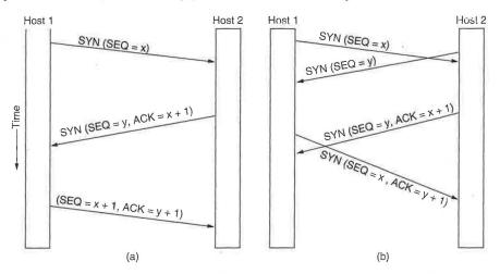
Figure 6-31. (a) TCP connection establishment in the normal case. (b) Call collision.
