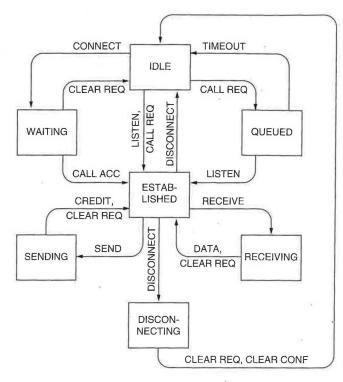
Figure 6-22. The example protocol in graphical form. Transitions that leave the connection state unchanged have been omitted for simplicity.
