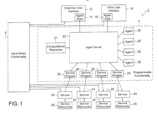
As shown in network system 2 of Figure 1, above, "agent server 20 controls, coordinates, and otherwise manages the overall operation of programmable functionality component 4" and, further, "may invoke, initiate, or execute various routines, processes, objects, and the like." *Id.* at 7:51–55. "For example, when a user wishes to interact with network system 2 via graphical user interface 12, agent server 20 may cause web pages to be downloaded to
