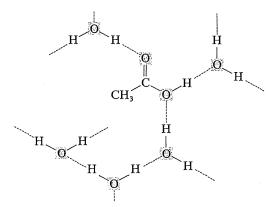
acetic acid, hydrogen bonded to water molecules in aqueous solution
