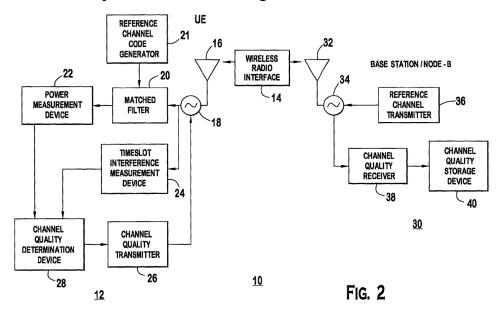
Figure 2 shows a block diagram illustrating a UE and a base station for implementing channel quality measurements for downlink resource allocation.
