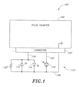
Figure 1 illustrates a schematic of a pulse oximeter system. *Id.* at 2:30–31. The wavelengths of light pass through the flesh of a patient to be detected by
