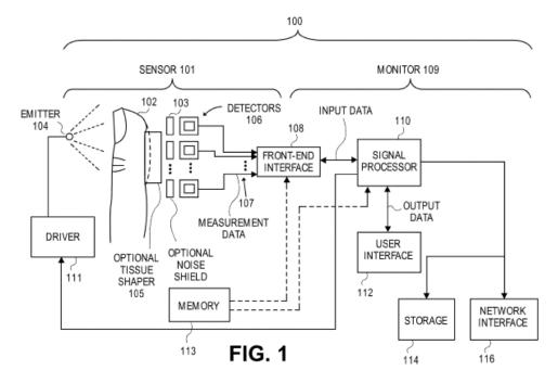
Figure 1 illustrates a block diagram of data collection system 100 including sensor 101 and monitor 109. *Id.* at 11:36–47. Sensor 101 includes optical emitter 104 and detectors 106. *Id.* at 11:48–52. Emitters 104 emit light that
