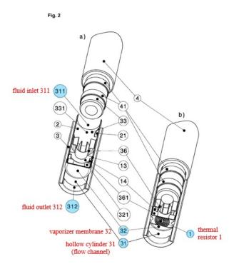
Annotated Fig. 2 above highlights the location of the electronic cigarette's "fluid inlet" (311), "hollow cylinder"/"flow channel" (31), "thermal resistor" (1), "vaporizer membrane" (32), and "fluid outlet" (312). *Id.*, Fig. 2, Table 1.
