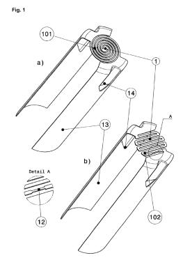
Figure 1 shows two variants of a heating device that includes thermal resistor 1, where the heating device is produced from a single piece of metal foil. Ex. 1001, 7:21–25. In Figure 1a, thermal resistor 1 takes the form of dual coil 101, and in Figure 1b, thermal resistor 1 takes the form of sinuous line 102. *Id.* at 7:26–28.
