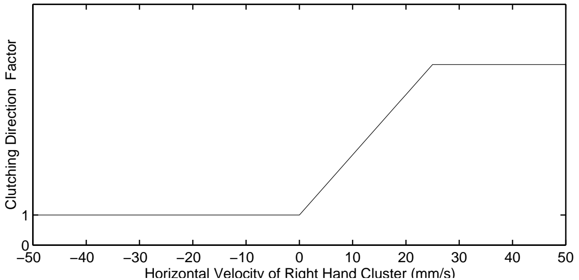
Figure 4.37: Hand clutching direction factor versus the average of the right hand's horizontal contact velocities.
