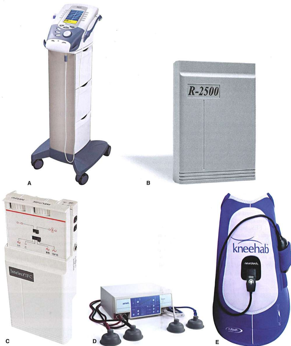
FIGURE 13-1 A: Cabinet-type, line-powered, multi-current stimulator mounted on cart, capable of generating Russian, interferential, and pulsed biphasic currents. Portable, battery-powered Russian ( B ) and interferential ( C ) stimulators. D: Cabinet-type, line-powered, interferential with vacuum unit, to which is attached a pair of suction electrodes. E: Newer, one size fits all, battery-powered, garment-based electrical stimulator designed specifically for the quadriceps muscle. (A–C: Courtesy of DJO Global; D: Courtesy of Astar; E: Courtesy of Neurotech Bio-Medical Research Ltd.)
