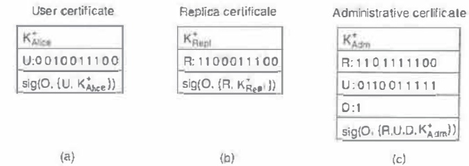
Figure 10-21. Certificates in Globe: (a) a user certificate, (b) a replica certificate, (c) an administrative certificate.
