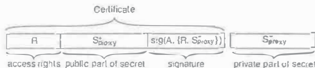
Figure 9-38. The general structure of a proxy as used for delegation.
