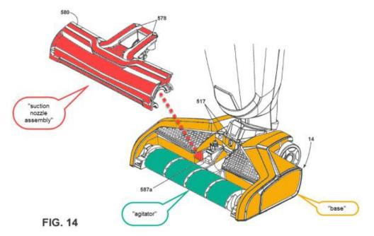
As shown above, the vacuum cleaning apparatus comprises a suction nozzle assembly, a base, and an agitator. The suction nozzle assembly includes, for example, a nozzle housing, nozzle cover, fluid delivery channels, fluid dispensers, spray tips, a nozzle cover, and wipers. *Id.* at 8:11–34. Bissell's (Prelim. Resp. 7, reproduced in Pet. Reply 12) annotated Figure 8 of the '455 patent, reproduced below, depicts the exemplary parts of the suction nozzle assembly.
