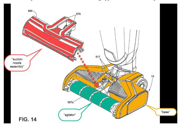
As shown above, the vacuum cleaning apparatus comprises a suction nozzle assembly, a base, and an agitator. The suction nozzle assembly includes, for example, a nozzle housing, nozzle cover, fluid delivery
