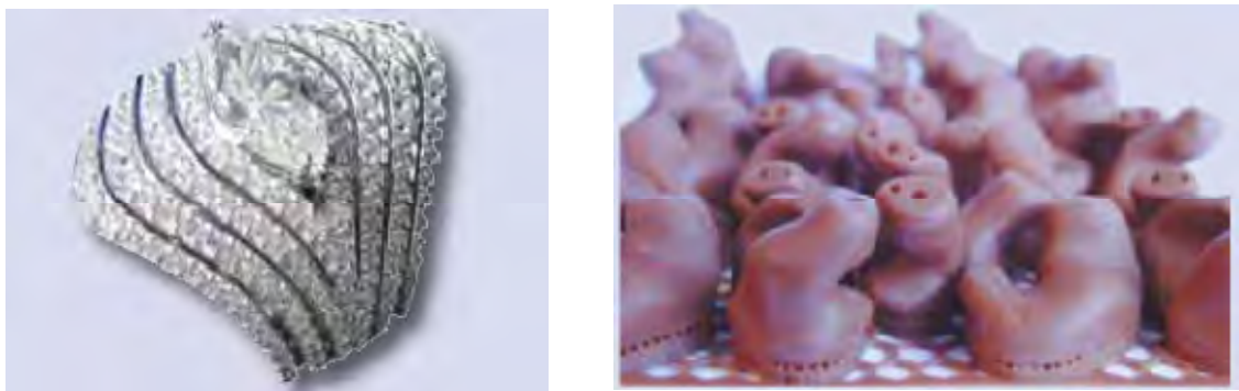
Figure 2-11: Production of Jewellery and Hearing Aid by Envisiontec Perfactory©
