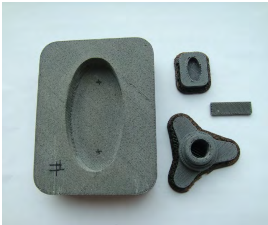
Figure 7-10: Fused Deposition Modelling of ABS/Iron Composites in FDM3000
