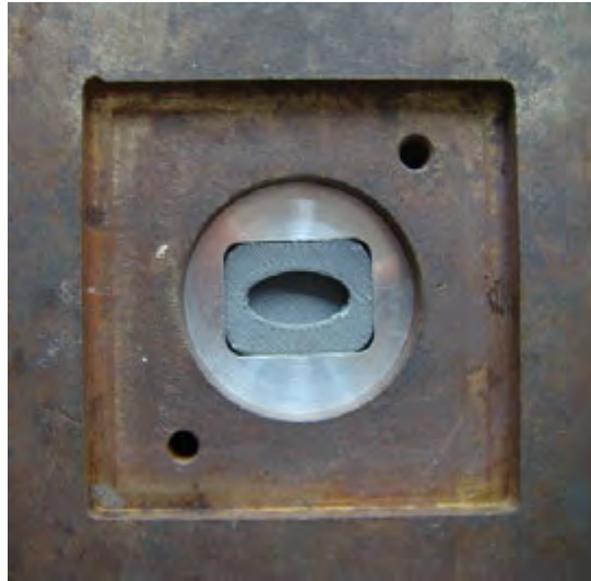
Figure 7-13: Mini tool insert fabricated on FDM fitted into steel blade for injection moulding
