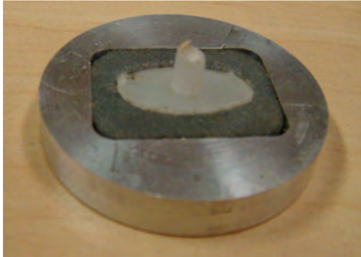
Figure 7-15: Polypropylene part made in mini injection moulding process on an ABS/Iron tool inserts
