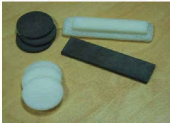
Figure 3-9: Test samples produced on FDM3000 from the new Iron/ABS composite and unfilled ABS material (white).
