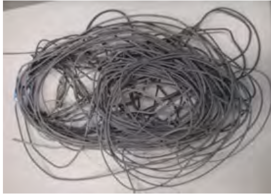
Figure 3-8: FDM filament produced from Iron/ABS composite material.
