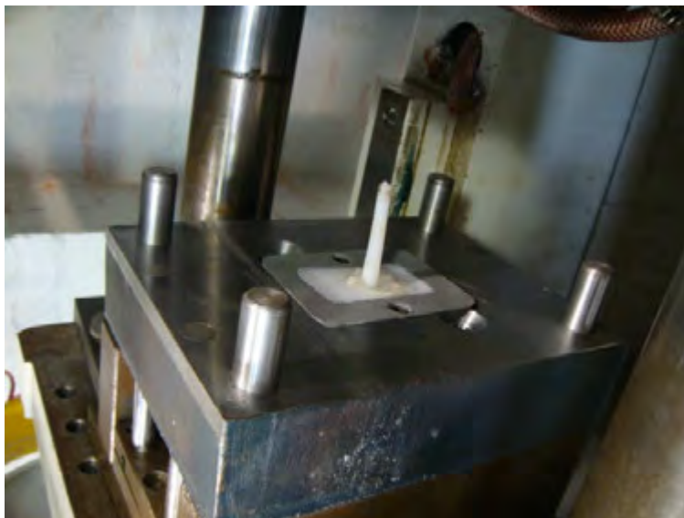
Figure 7-19: HDPE part produced by injection moulding into Iron/ ABS tool insert made on FDM platform
