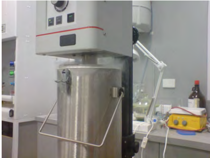
Figure 3-3: Cryogenic grinding of ABS polymer
