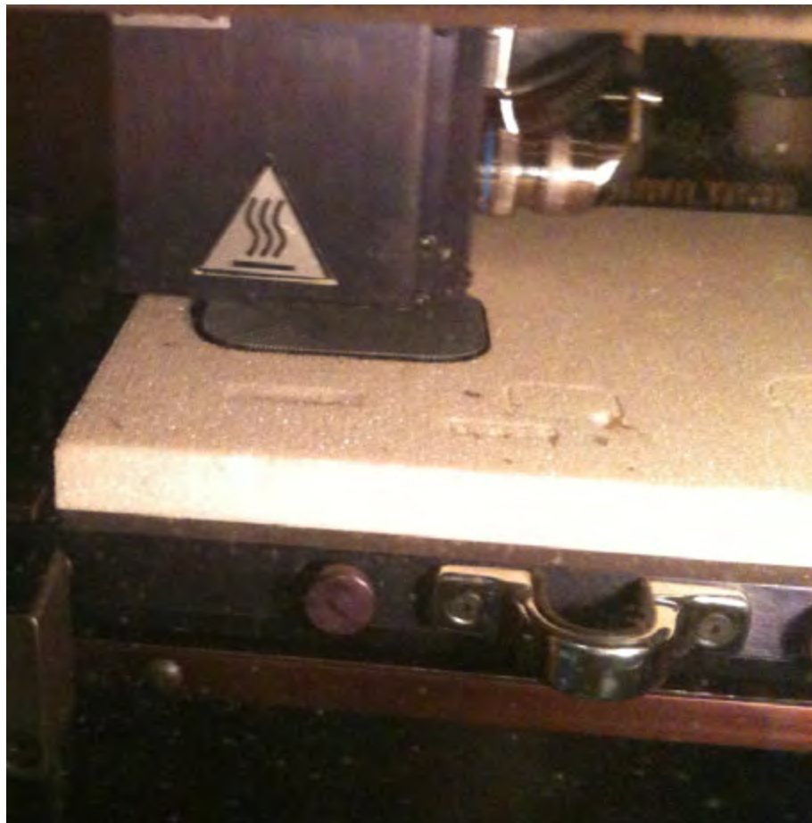
Figure 7-3: Fused Deposition Modelling of ABS/Iron Composites in FDM3000
