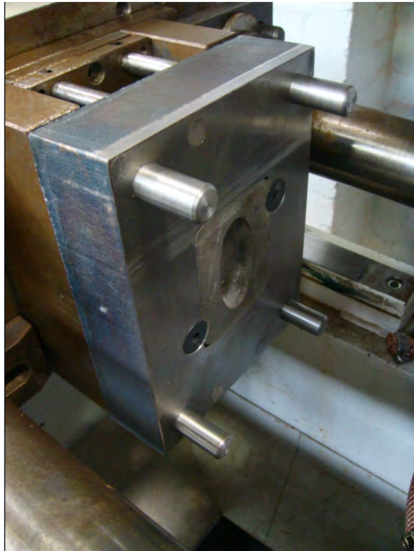
Figure 7-16: Injection moulding cavity insert of ABS/Iron composite fitted into the injection mould base
