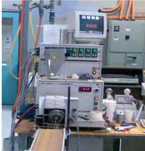
Figure 3-4: Single screw extrusion of the ABS-Fe filaments
