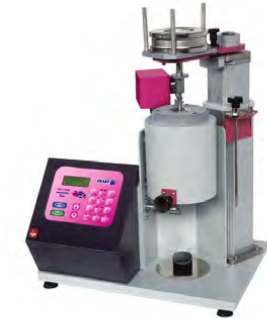
Figure 4-7: CEAST Melt Flow Indexer
