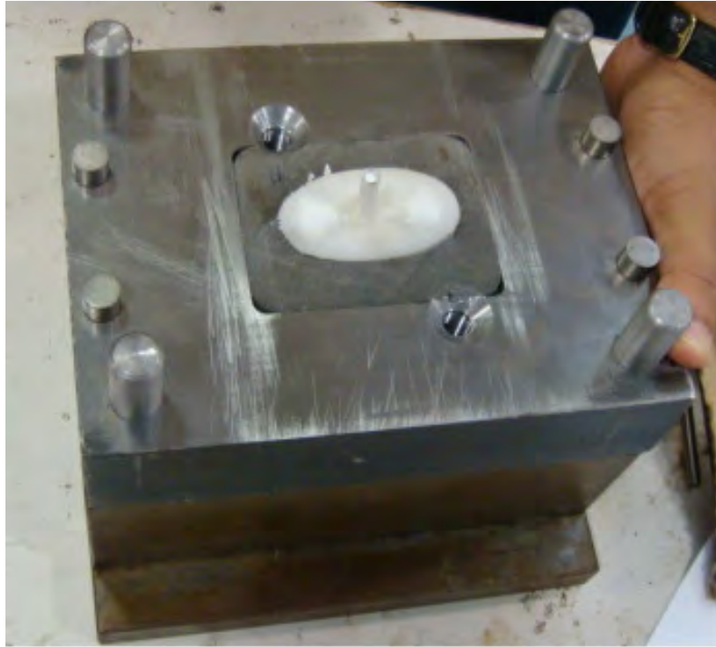
Figure 7-18: PP part produced by injection moulding into Iron/ ABS tool insert made on FDM platform.
