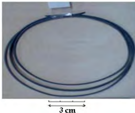
Figure 6-2: FDM filament produced from Iron/ABS composite material
