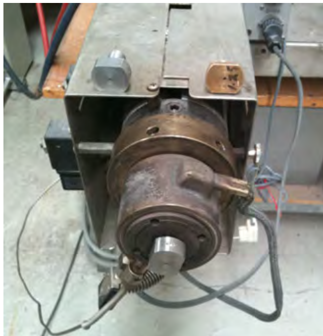
Figure 3-7: Long land length die for suppressing extrusion swell
