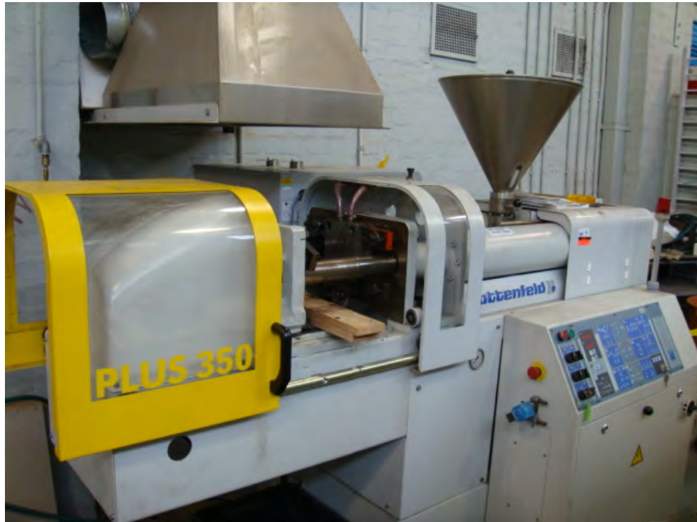
Figure 7-17: Battenfeld Injection Moulding machine was fitted with metal/polymer tool inserts
