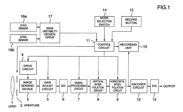
In Figure 1, above, depicting an embodiment of an electric camera, "light coming from the lens 1 through the aperture 2 is focused on a light receiving surface of the image sensing device 3 where it is converted into an electric signal." *Id.* at 4:31–34. Image sensing device 3 is of a CCD [charge-coupled device] type, with pixels formed from photodiodes and arranged in a grid pattern. *Id.* at 4:34–38, Fig. 2.
