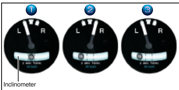
Figure 12-8. In a coordinated turn (instrument 1), the ball is centered. In a skid (instrument 2), the rate of turn is too great for the angle of bank, and the ball moves to the outside of the turn. Conversely, in a slip (instrument 3), the rate of turn is too small for the angle of bank, and the ball moves to the inside of the turn.
