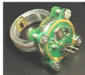
Figure 1: The photograph of the finger ring sensor. The size of the circuit board on top of the ring is 0.8 by 0.8 inch.
