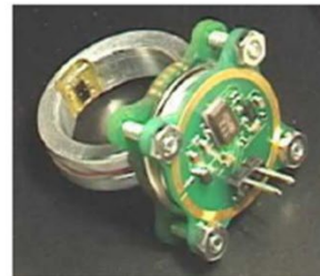
Figure 1: The photograph of the finger ring sensor. The size of the circuit board on top of the ring is 0.8 by 0.8 inch.
