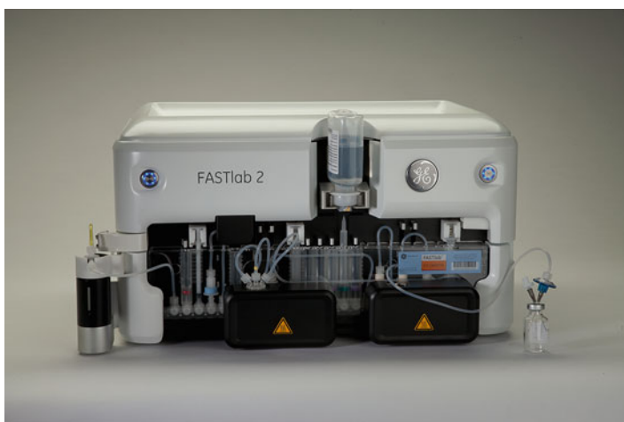
Fig. 8.2 Automated synthesis box, FASTlab2, from GE Healthcare (Courtesy of GE Healthcare)
