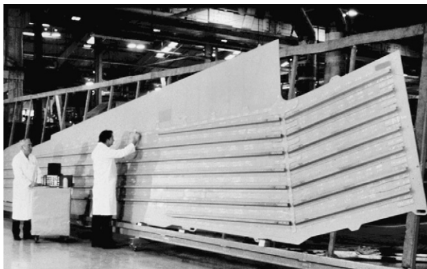
Figure 13.12 Redux-bonded wing assembly in the BAE SYSTEM's RJ 80 (formerly the BAe 146).
