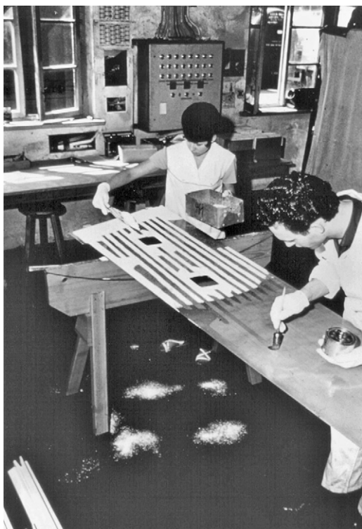
Figure 13.5 Application of Redux liquid and powder adhesive to an airframe component.
