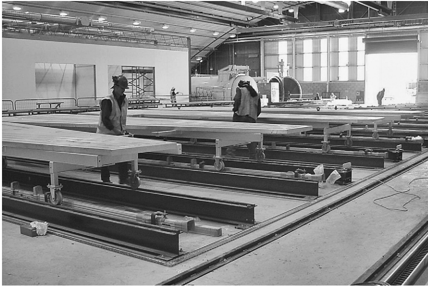
Figure 13.52 Autoclave bonding shop; railway system to take the tools to the autoclave (courtesy of BAE SYSTEMS, Broughton).
