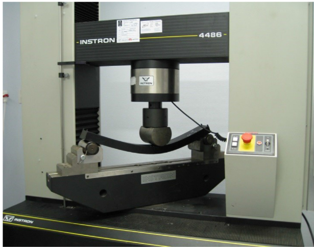
Figure 1.6 Picture of a three point flexural or bending test being done in an Instron universal testing machine [3].
