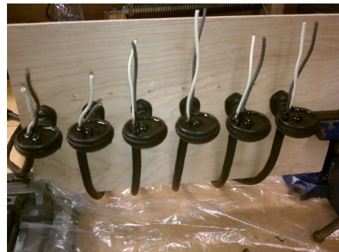
Figure 4: Custom cable potting for thrusters
