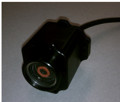
Figure 11: Camera pressure vessel with assembled Point Grey camera.
