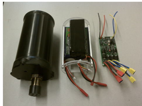
Figure 10: Battery pod pressure vessel and internal
